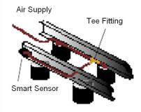
Smart Scale installs quickly. Bolt the Smart Sensor to the vehicle's frame, use the supplied tee-fitting to access the air line behind the height control valve, and you're ready to calibrate your scale.
